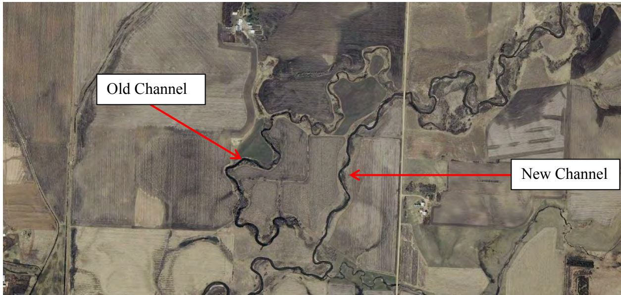
Figure 56. Historical channel cutoff on Kanaranzi Creek upstream of study site. The old channel measures out to be 10,708 feet, while the current channel measures out at 3,319 feet; a difference in 7,389 feet or 1.4 miles. Areas like this should be restored into their old channel in order to achieve higher water storage potential and maintain channel stability.
