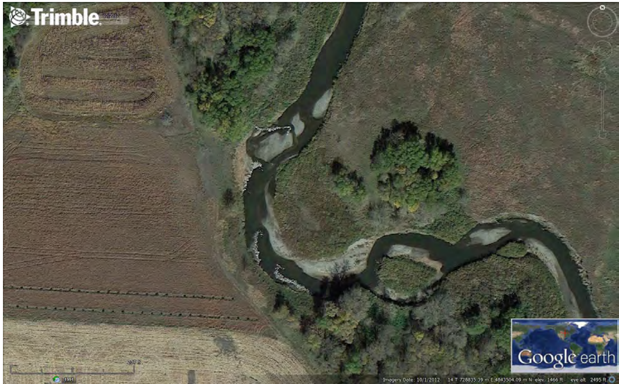
Figure 57. Aerial photo of a J-hook project on the Rock River that was designed outside of specifications made for J-hooks. This has resulted in issues with bedload deposition downstream of the 1st J-hook. Photo courtesy of Google Earth.
