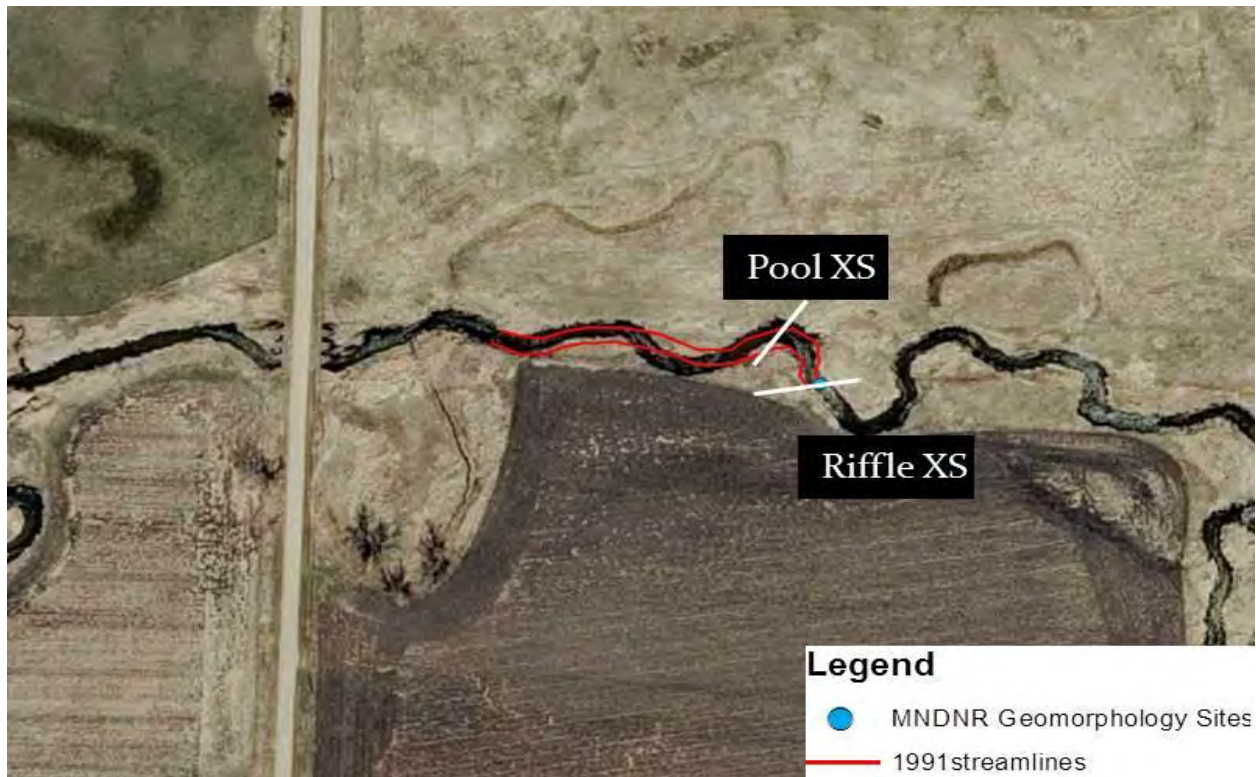
Figure 40. Aerial photo of the survey reach with labeled cross section locations and 1991 stream lines.
