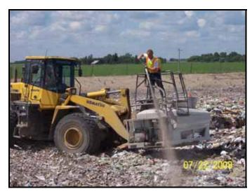
Applying a spray-on cover material
