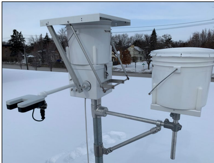
Figure 2. The N-CON automatic wet/dry atmospheric sampler on site in St. Louis Park.
