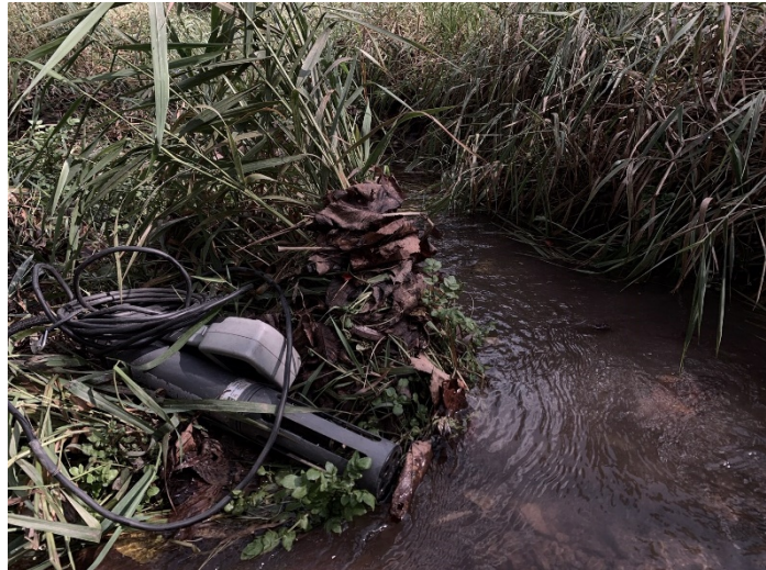
State agencies deployed equipment to measure water quality parameters, such as dissolved oxygen levels, as part of the response to the fish kill on Gavin Brook.
