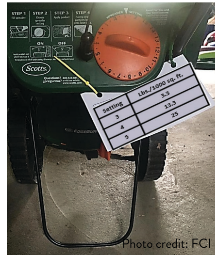
Figure 18: Calibration card zip tied to push spreader.
