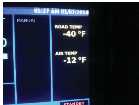
Figure 15: Mirror mounted pavement temperature sensor and temperature sensor display inside a vehicle's cab.
