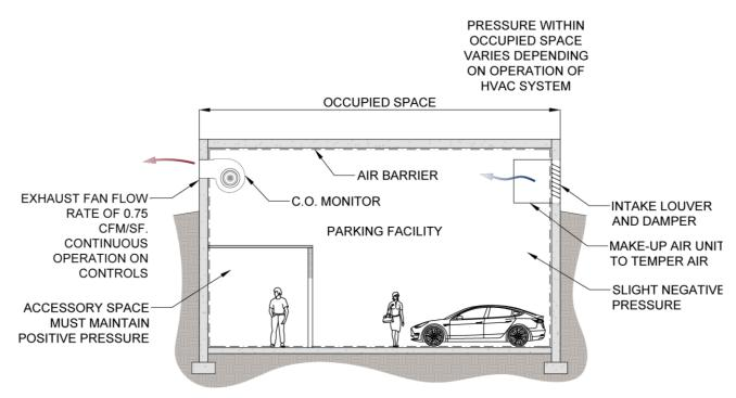
Figure 5.1 Typical Parking Facility with Full-Time (Continuous) Ventilation
