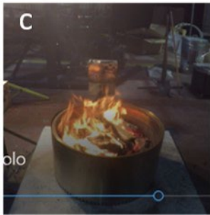
Figure 3. Burn phases of firepit testing a) ignition fuel bed, b) ignition, c) burn-up phase, d) steady burn phase, and e) burn-down phase.
