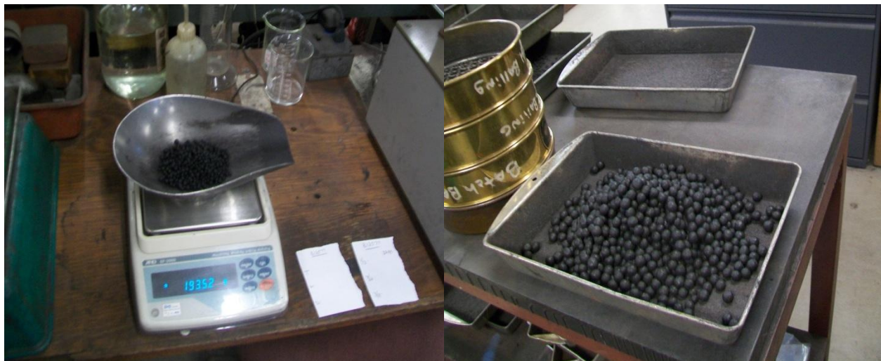
Figure 2. Pictures showing a) green ball “seeds” b) Sieved green balls.
