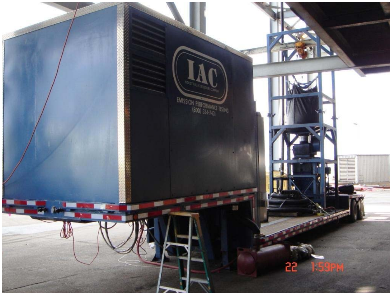
Figure 2. Sorbent injection trailer with the bulk bag lifter assembled and the bulk bag in place. The IAC box in the foreground houses the blower and compressor that provide the pressurized air to conveying the sorbent into the flue gas duct.
