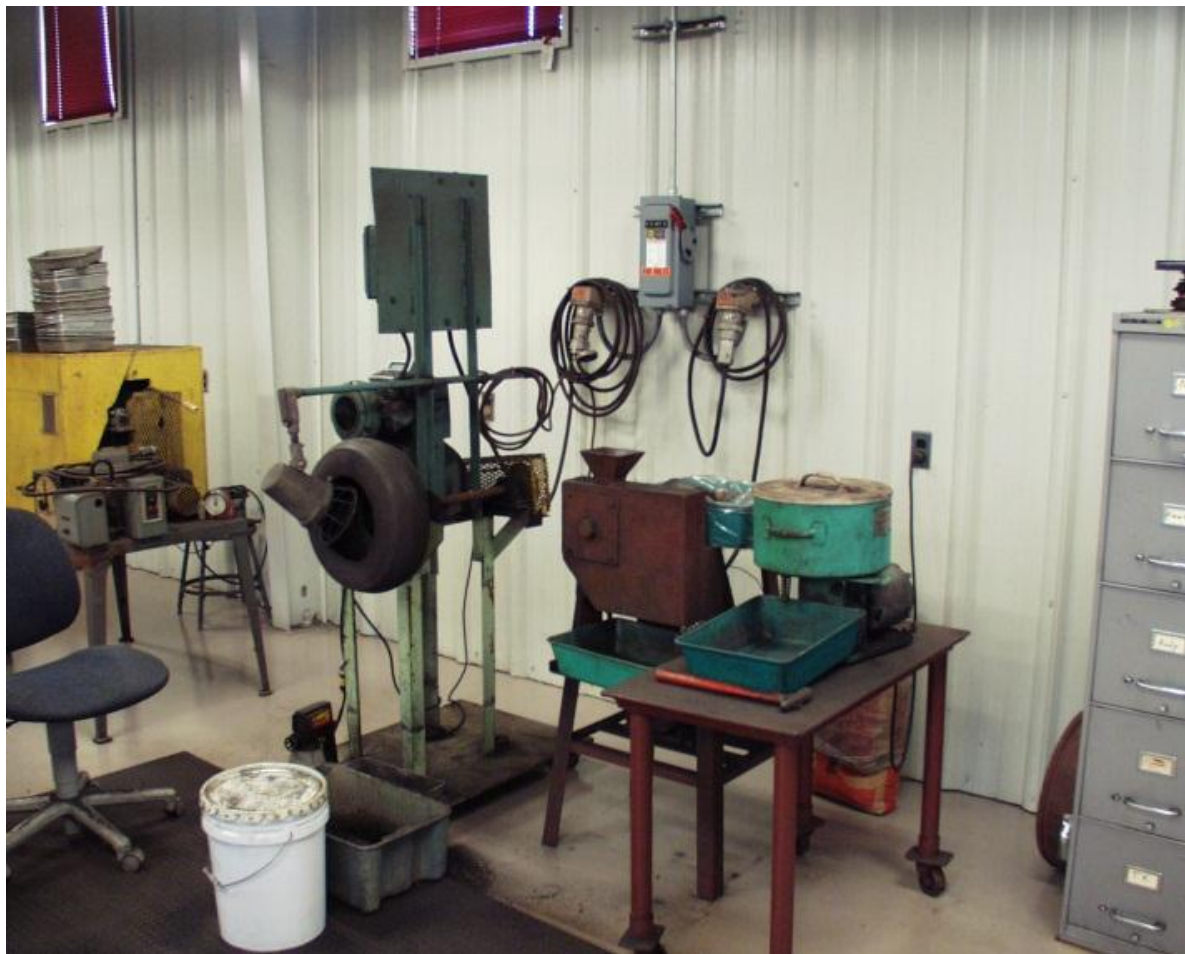
Figure 1. Batch balling test equipment and arrangement
