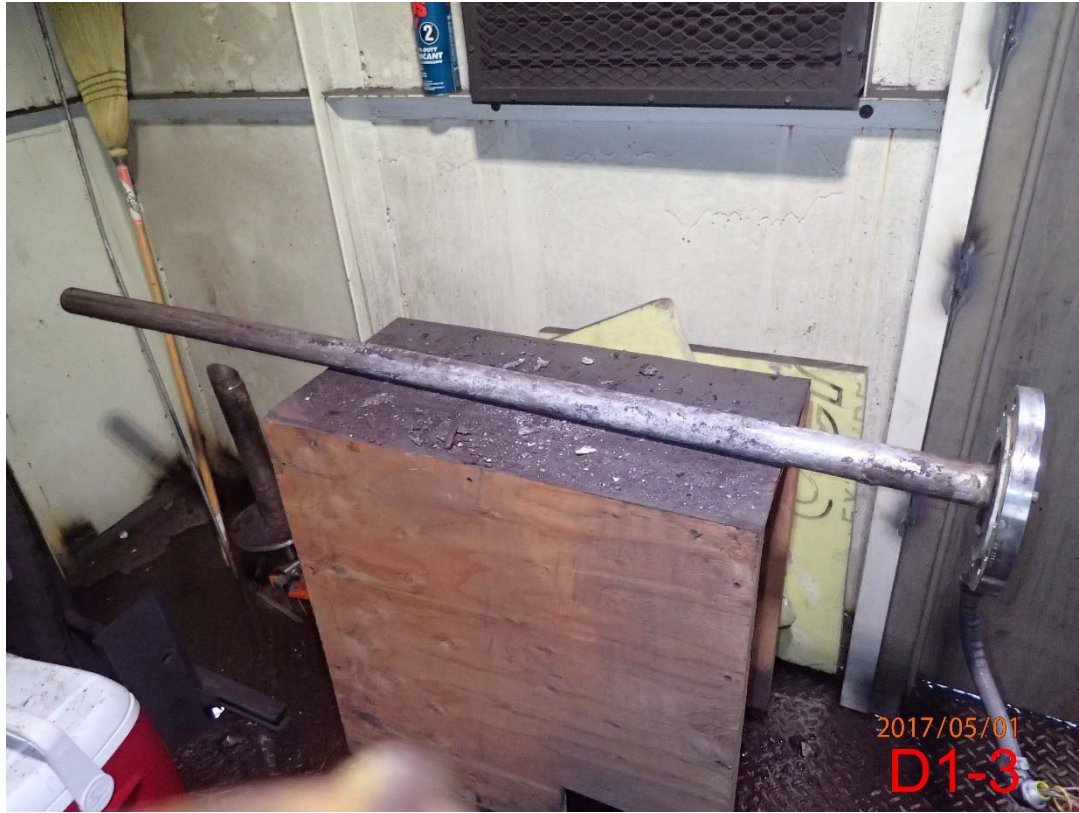
Photo 93 Stack D CEMS Probe (2)
