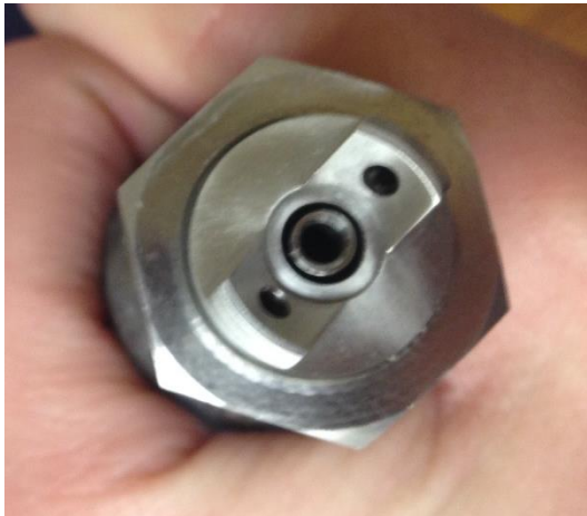
Injection nozzle before test
