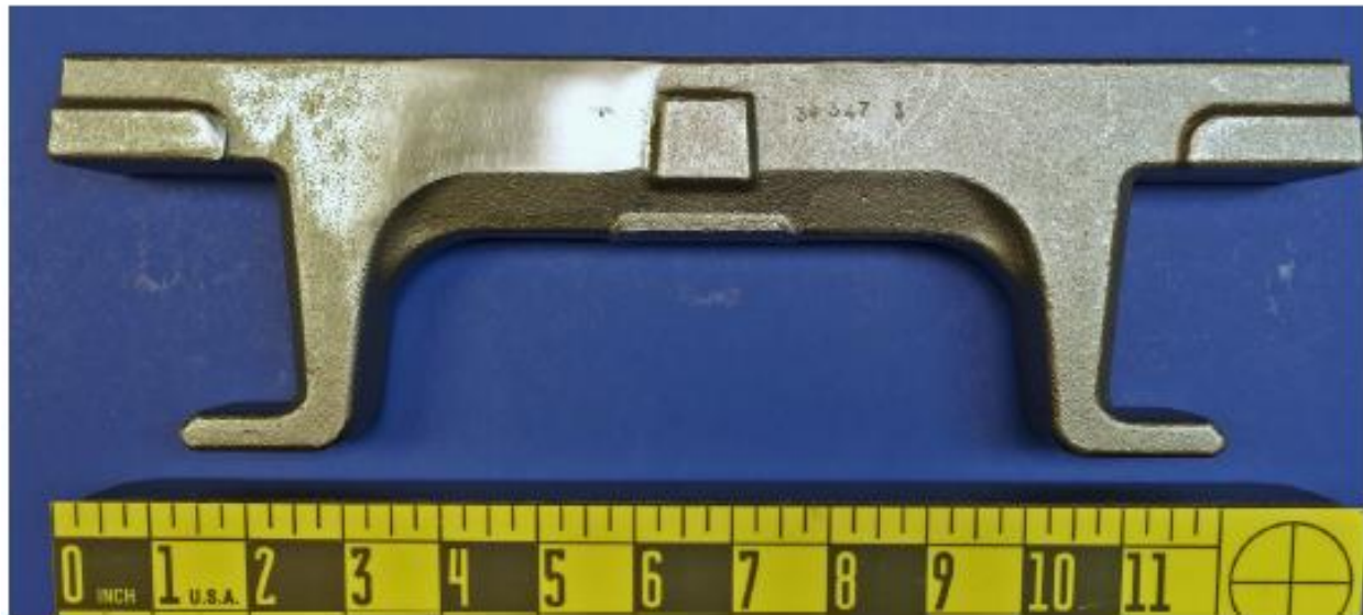
Figure 3. Furnace grate showing area that was ground and stamped ID.
