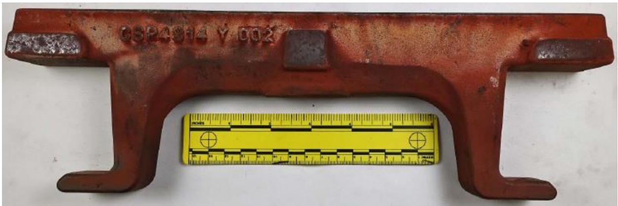
Grate Bars after test (photo courtesy of Corrosion Testing Laboratories, Inc.)
