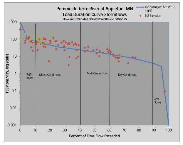
Figure 6.2: Load Duration Curve with Stormflow Samples
