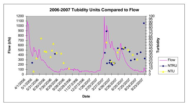
Figure 3: NTU and NTRU Turbidity units compared by date and correlated to flow
