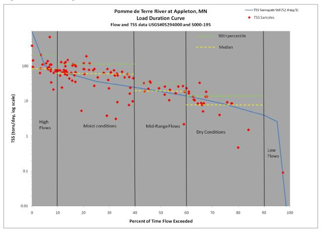
Figure 6.1: Loading Duration Curve for PdT River
