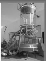
Selective Catalytic Reduction (SCR) processes are modeled to ensure that the catalyst is effective and catalyst life is extended for as long as possible. Proper mixing of flue gas and good flow and velocity profile are required to prevent ammonia slip and ensure that  $NO_{\chi}$  emissions are minimized.
