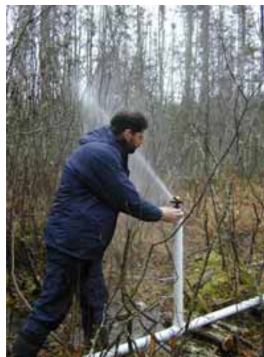
Ed Swain adjusting experimental sulfate addition to a wetland
