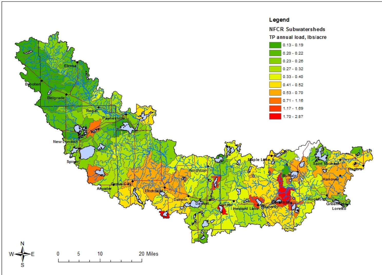
Figure 5. Total phosphorous loading by sub-watershed in the NFC watershed
