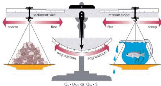
Figure 11: Generalized relationship of stream stability (Rosgen)
