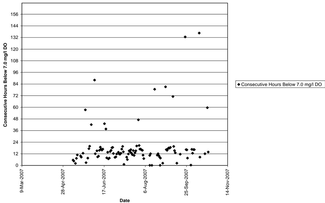
**Figure 25. Consecutive hours below DO of 7.0 mg/l at McKusick, 2007 monitoring data, Brown's Creek**
