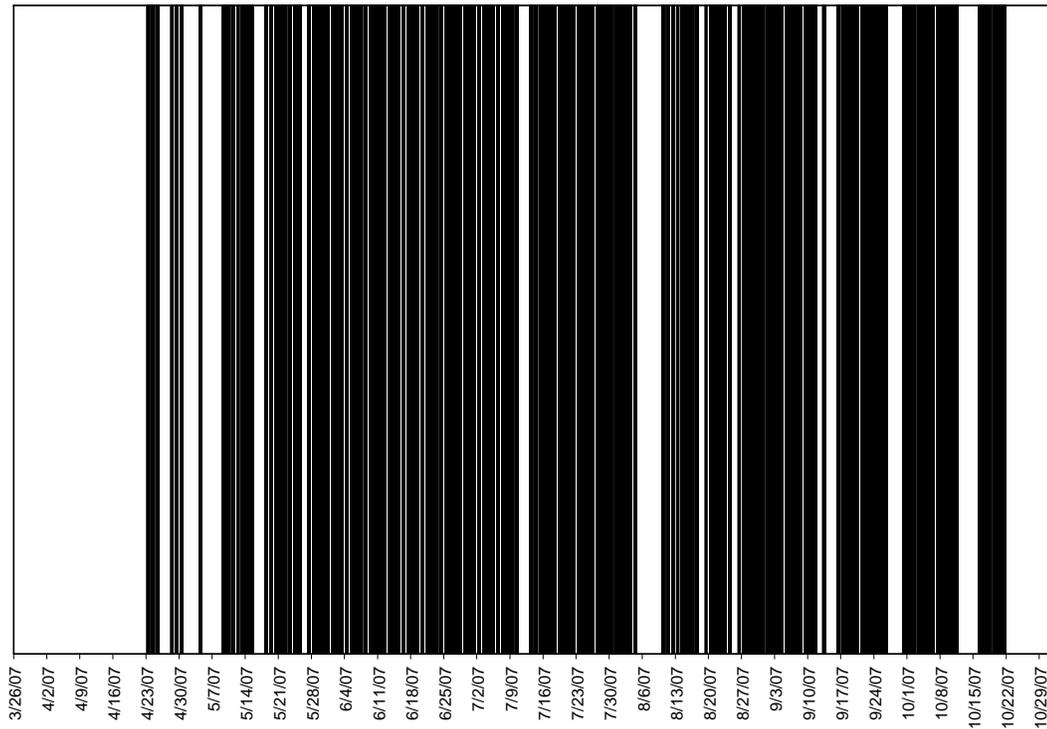
**Figure 18. Frequency of 15 minute periods below DO levels of 7.0 mg/l, McKusick, Brown's Creek.**
