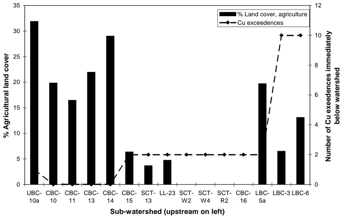
**Figure 56. Percent landscape covered by homes in sub-watersheds of Brown's Creek plotted against the non-cumulative number of times copper levels exceeded standards at monitoring stations immediately downstream (upstream on the left).**
