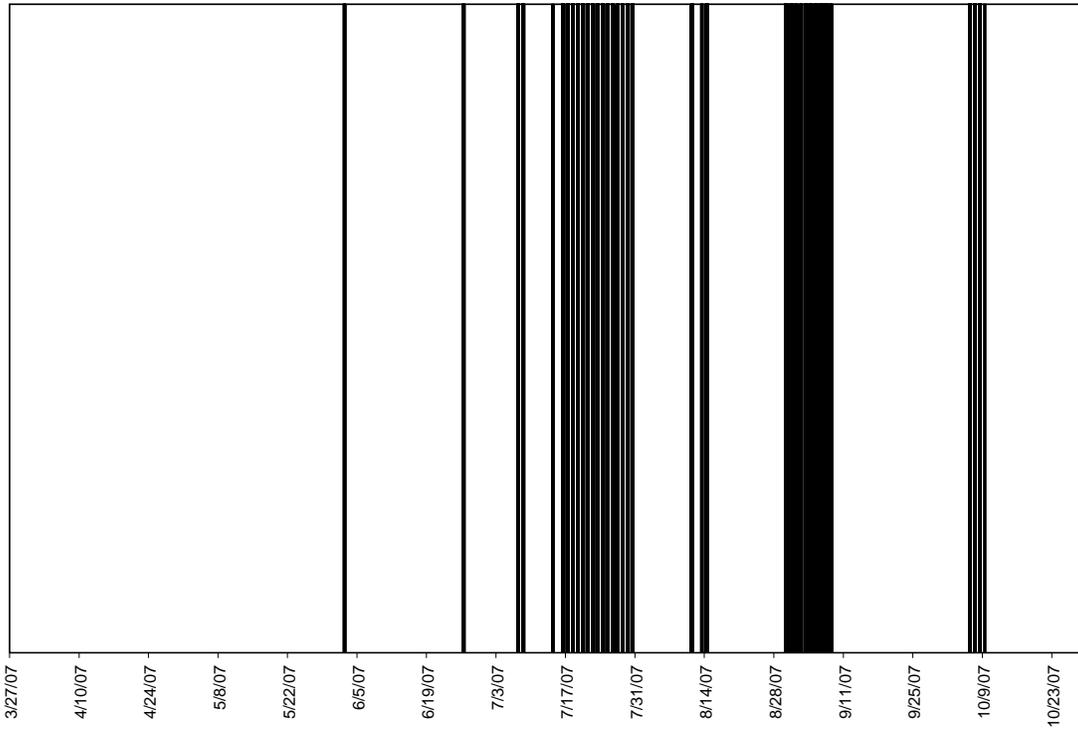
Figure 19. Consecutive hours below DO of 5.0 mg/l at 110<sup>th</sup> St., 2007 monitoring data, Brown's Creek. Data not available from 7 August to 20 September 2007.
