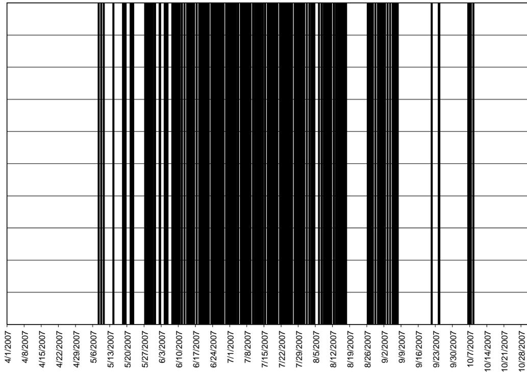
**Figure 40. Frequency of 15 minute periods above brown trout threat temperature (65° F, 18° C) at McKusick, Brown's Creek, 2007.**
