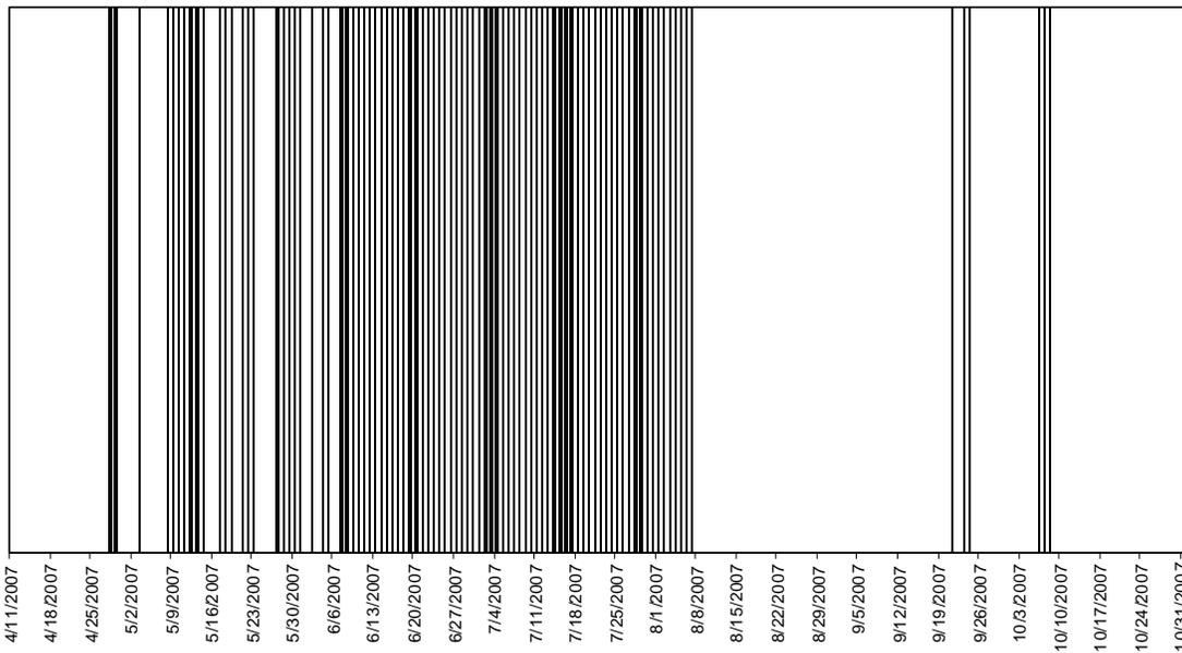
Figure 38. Frequency of 15 minute periods above brown trout threat temperature (65° F, 18° C) at Gateway, Brown's Creek, 2007.
