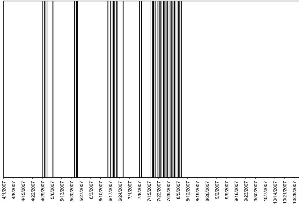
**Figure 15. Frequency of 15 minute periods below DO levels of 7.0 mg/l, Gateway, Brown's Creek.**
