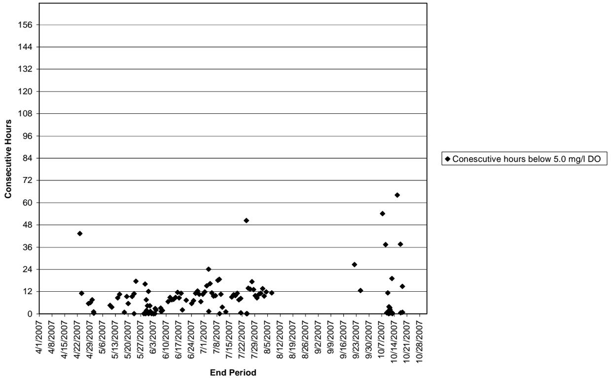
Figure 20. Consecutive hours below DO of 7.0 mg/l at 110<sup>th</sup> St., 2007 monitoring data, Brown's Creek. Data not available from 7 August to 20 September 2007.
