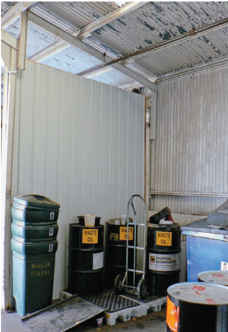
This facility is collecting and storing waste fluids under cover and with containment to avoid exposing pollutants to stormwater.
