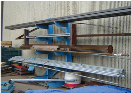
Raw materials like steel, coated with oil or subject to corrosion, need to be sheltered to qualify for the No Exposure Exclusion.
