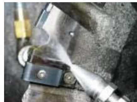
Spraying CO 2 “snow” on a part to cool and lubricate. No mess, no fuss, no post-machining clean-up needed.
