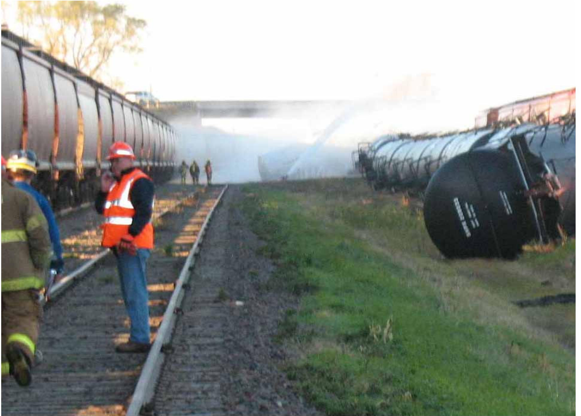
Workers sprayed a water mist to prevent the release from the broken tank.
