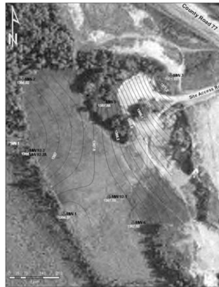
Figure 5. Highway 77 Sanitary Landfill Ground Water Flow Direction August 2006
