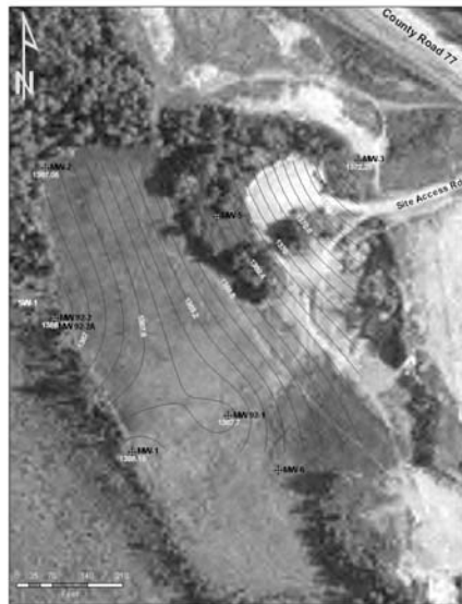
Figure 4. Highway 77 Sanitary Landfill Ground Water Flow Direction August 2005
