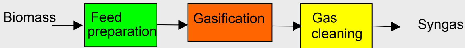
Biomass Syngas Platform
